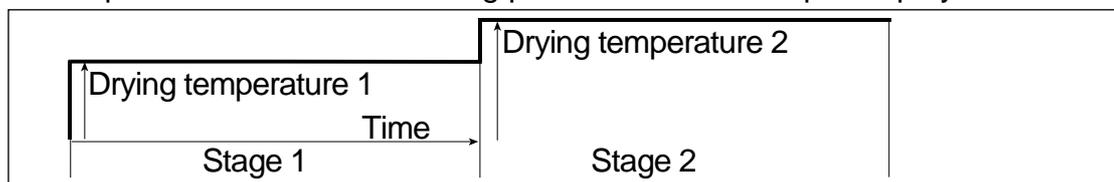
"Temperature 1" can be set higher than "temperature 2" in step drying.
