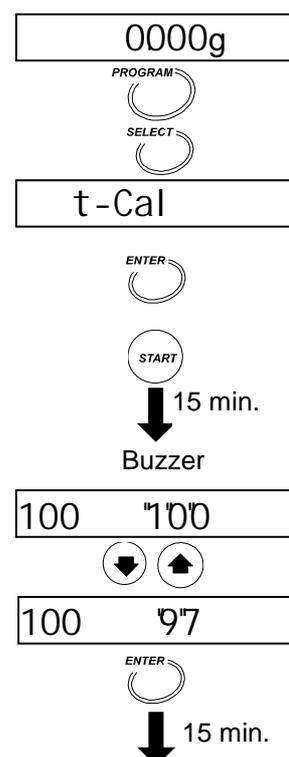
10. After fifteen minutes, the buzzer sounds and the display blinks 160°C. Adjust the blinking value to the thermometer value using the ↓ or ↑ key. (Example: 162°C)
